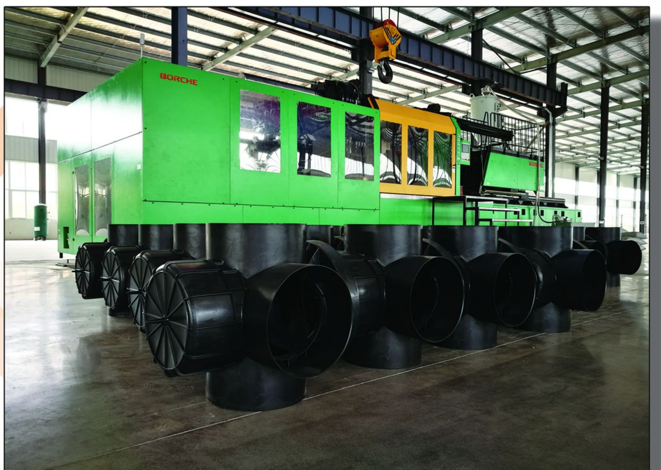
1,500t and 2,500t high volume injection machine in factory, competent in most mold samplings and adjustments.
